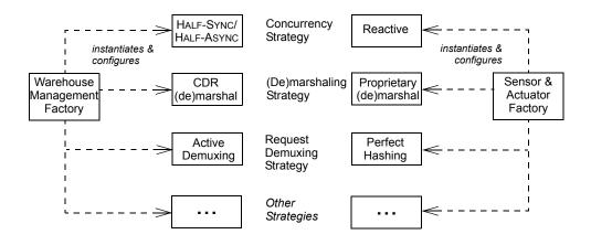
Our use of ABSTRACT FACTORY simplifies ORB maintenance and configuration by consolidating groups of ORB strategies with multiple alternative implementations that must vary together to ensure semantic compatibility for different warehouse management process control system subsystems.
