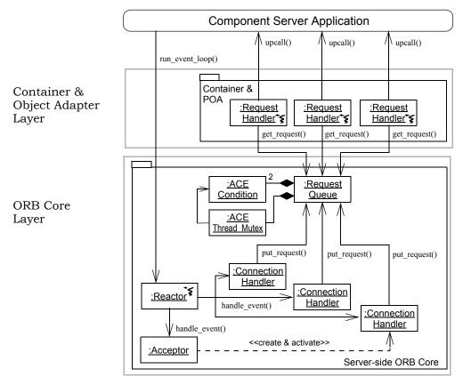
When a consumer thread running in the pool of RequestHandlers attempts to get a client request from an empty RequestQueue, the queue's get\_request() method atomically releases the monitor lock and the thread suspends itself on the not-empty monitor condition. It remains suspended until the RequestQueue is no longer empty, which happens when a ConnectionHandler running in the producer thread puts a client request into the queue.
