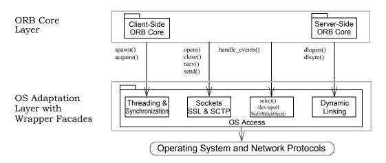
The encapsulation provided by the ACE WRAPPER FACADES provides a consistent object-oriented programming style and alleviates the need for the ORB to access the weakly-typed C system programming APIs directly. Standard compilers and language processing tools can therefore detect type system violations at compile-time rather than at run-time. As a result, much less effort is required to maintain the
