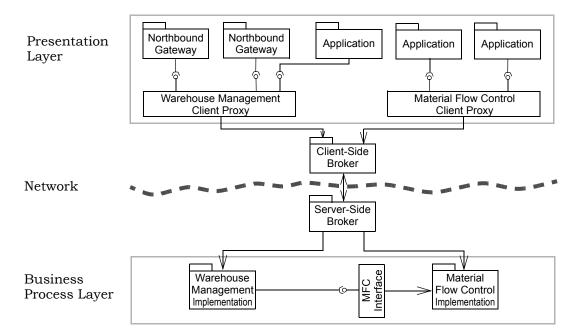
We implement the BROKER communication middleware for our warehouse management process control system using the *CORBA Component Model* (CCM) [OMG02]. The CCM is communication middleware that allows applications to invoke operations on components without concern for their location(s), programming language, operating system platforms, network protocols and interconnects, and hardware. CCM is essentially a language- and platform-independent variant of EJB. At the heart of the CCM
