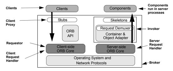
The client and server roles in the BROKER pattern represent the application-level clients and components in the OMG CCM reference model. The CLIENT PROXY (281) role is implemented by the ORB's Stubs, which provide access to the services offered by remote components. Stubs also shield clients and servers from the location and the implementation details of their remote communication partners, as well as from the specifics of the ORB implementation.
