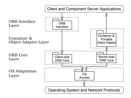
The diagram below illustrates the layered design for our CCM-based ORB:
