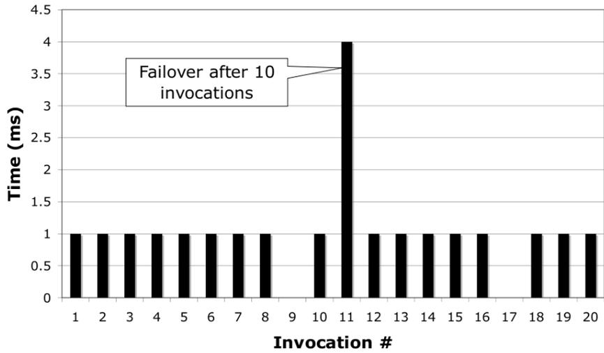
Figure 11: Single Fail over Latency Measurement
