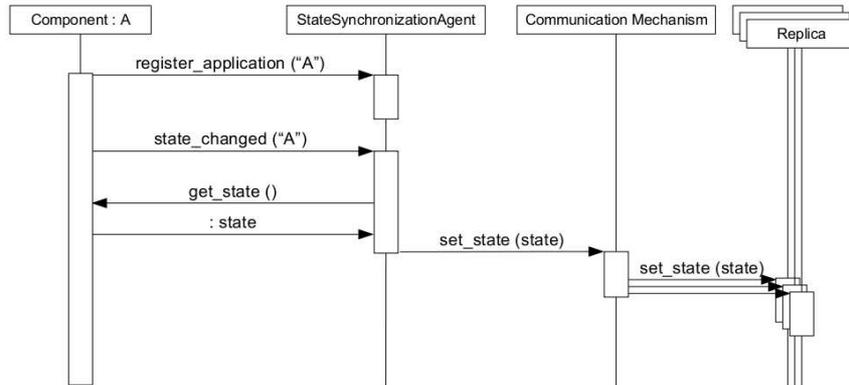
Figure 8: State transmission sequence based on a common interface
