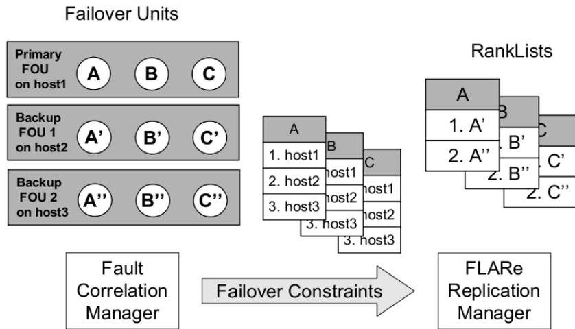
Figure 7: Interaction between FaultCorrelationManager and ReplicationManager through Failover Constraints
