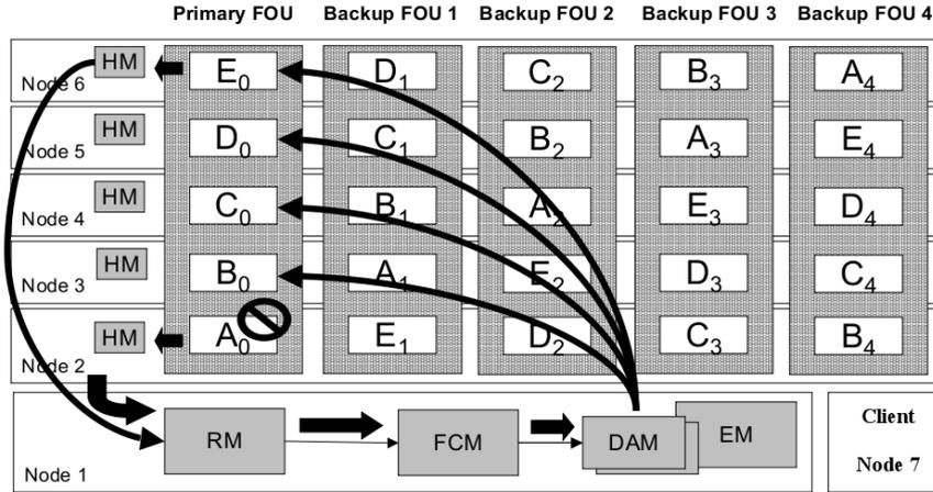
Figure 13: Setup for FOU Shutdown Latency Measurement
