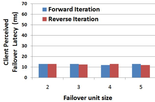
Figure 14: Client Perceived Fail over Latency When the Head Component Fails
