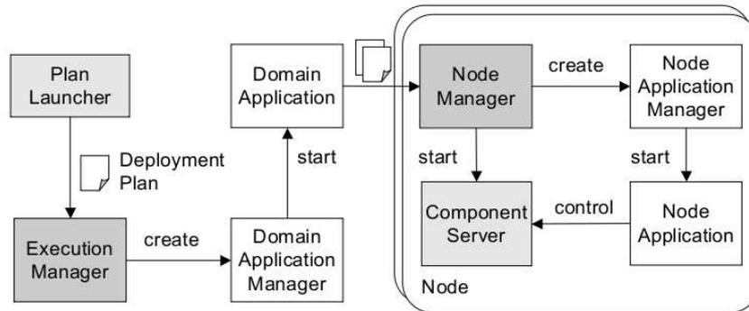
Figure 3: System Model for Component-based Deployment and Configuration
