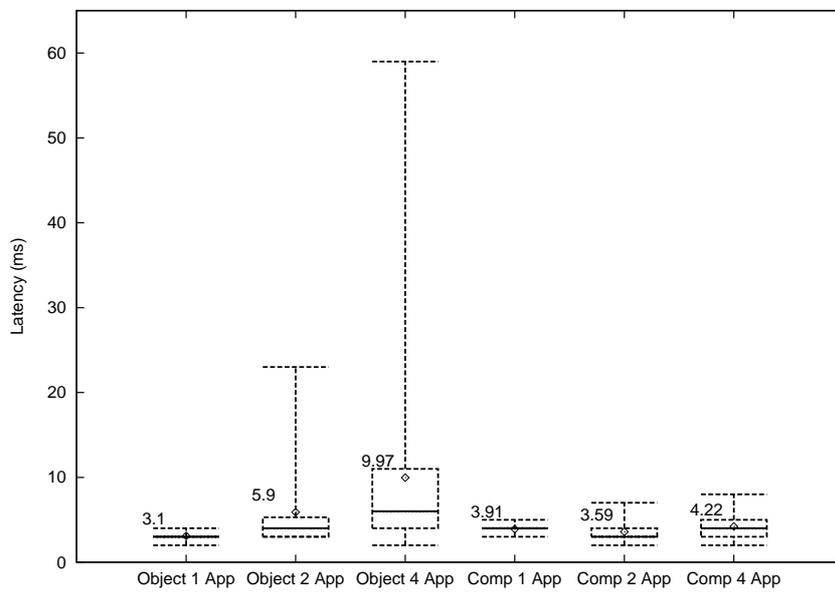
Figure 12: Results for Failover Latency Measurements
