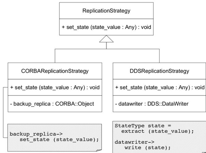
Figure 9: The Strategy Pattern Applied to State Synchronization
