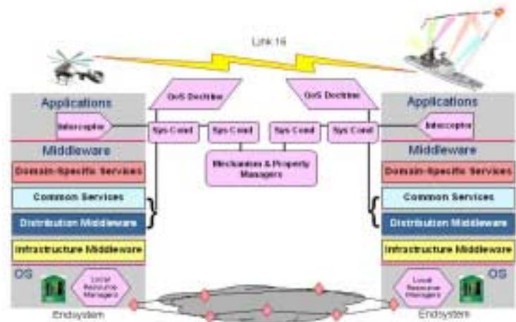
**Figure 3. Decoupling Functional and QoS Paths**
