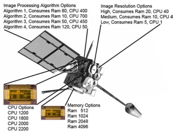
**Figure 1 Configuration Options of a Satellite Imaging System**
