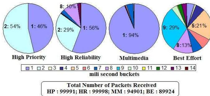
Fig. 12. Jitter Distribution under Different Network QoS Classes
