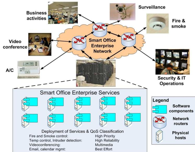
Fig. 1. Network Configuration in a Smart Office Environment
