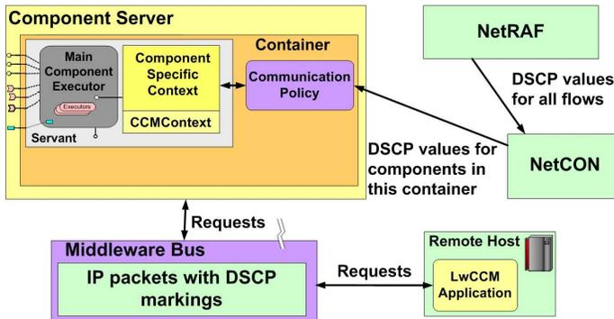
Fig. 6. NetCON's Container Auto-configurations
