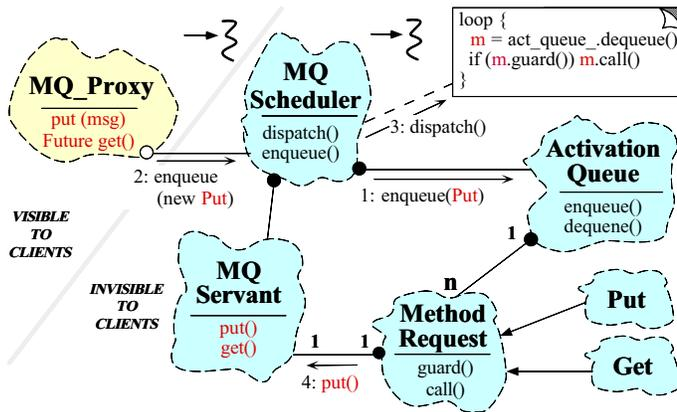
Figure 2: Implementing a Message Queue as an Active Object for Consumer Handlers
