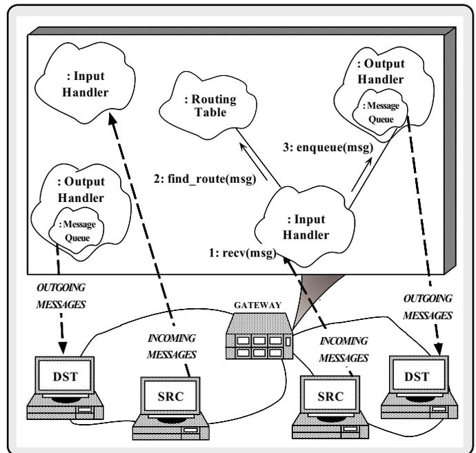
Figure 1: Connection-Oriented Gateway
