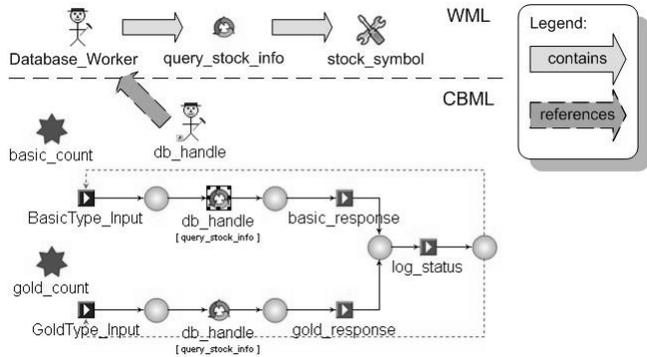
Figure 9. Example CBML model parameterized with WML actions.
