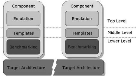
Figure 12. Code generation architecture for emulation.
