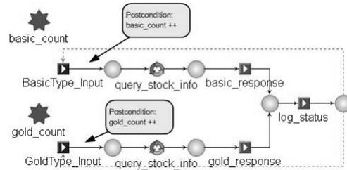
**Figure 6. Example CBML behavior model with variables.**
