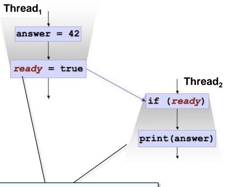
With proper use of synchronization Thread<sub>1</sub> will complete its writes to answer & ready before Thread<sub>2</sub> starts its reads of ready & answer
