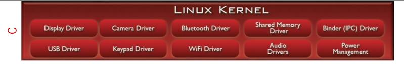
Android's local/remote inter-process communication (IPC) mechanisms mediate interactions between apps & system services
