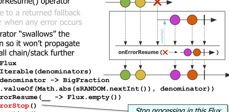
Stop processing in this Flux stream when an error occurs
