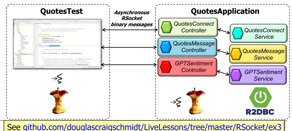
• This case study shows how an RSocket requester can exchange binary messages asynchronously with various controllers & services
