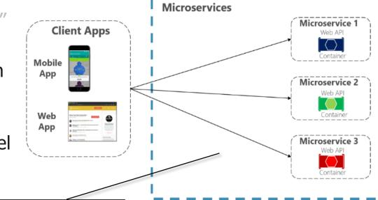
Each microservice has a public endpoint, e.g., with a different TCP port & host address
