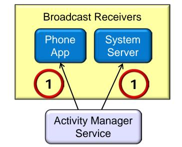
Normal – Sent with Context.sendBroadcast(), which is completely asynchronous
