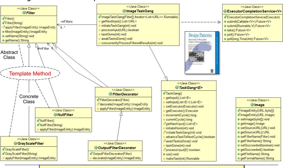
Template Method defines the skeleton of an algorithm in a method, deferring certain steps to subclass methods
