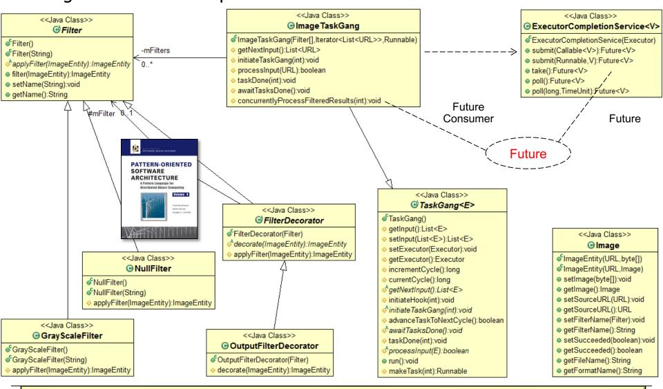
Future provides a proxy for a result that may not be available yet, allowing a program to continue execution without blocking until the result is needed
