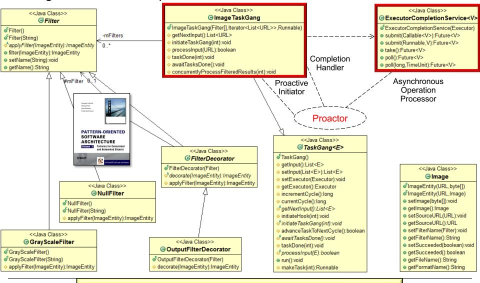
*Proactor* allows concurrent applications to efficiently process service requests & responses asynchronously
