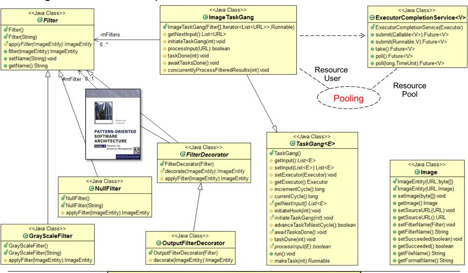
Pooling manages multiple worker threads& optimizes their acquisition & release
