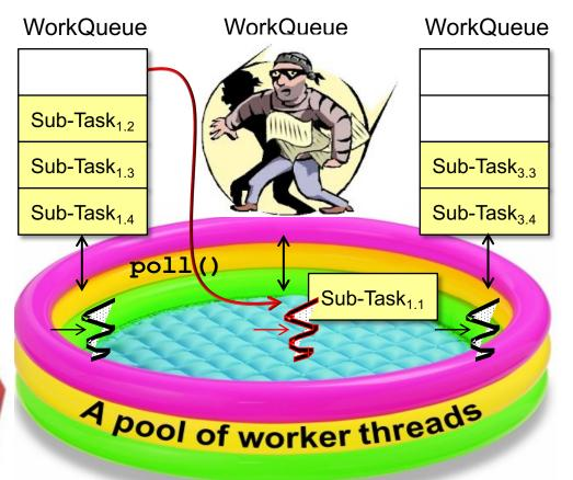
A parallel stream pushes larger chunks onto the deque before smaller chunks
