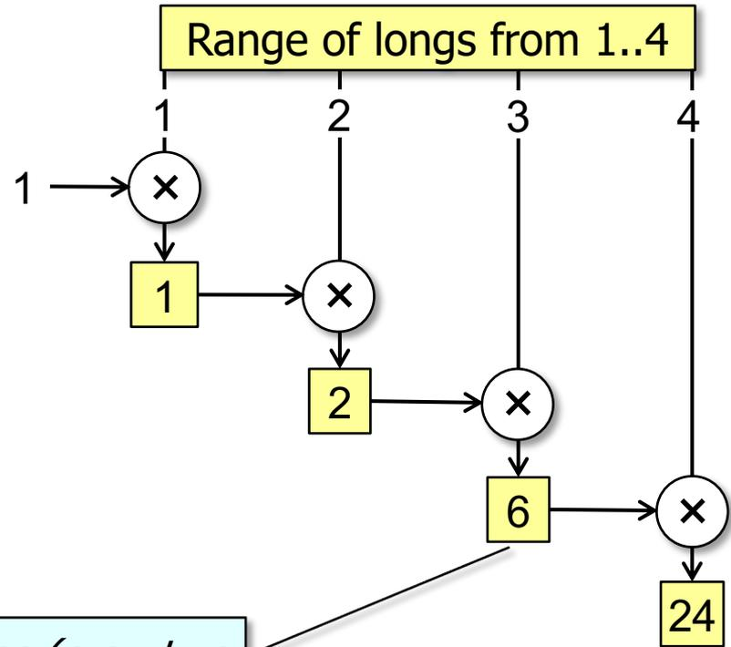
*reduce() combines two immutable values (e.g., two long, int, etc.) & produces a new immutable value*
