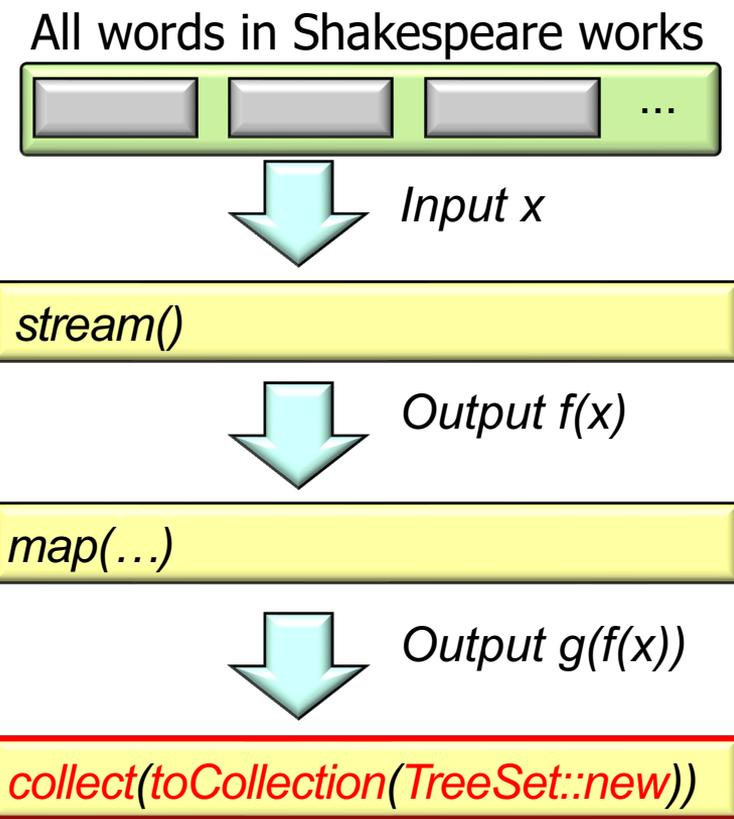
`toCollection()` creates a TreeSet container & accumulates stream elements into it
