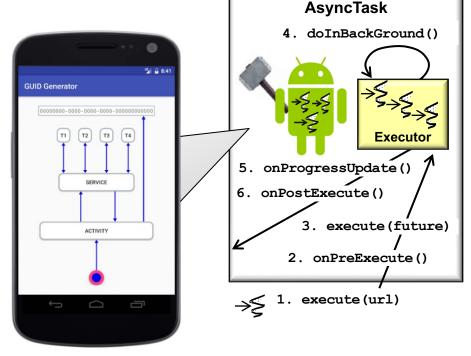
• e.g., Android's AsyncTask framework performs background operations & publishes results on the user-interface (UI) thread without having to manipulate threads and/or handlers
