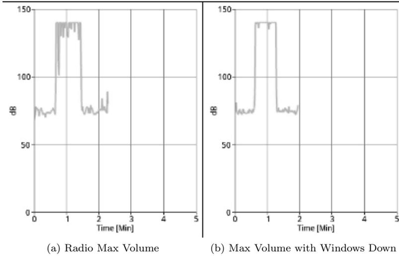
Fig. 11: Stereo Noise Levels During Highway Transportation
