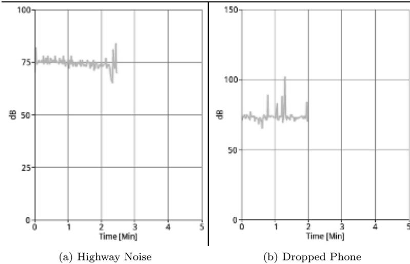
Fig. 9: Potential Noise Levels During Highway Transportation
