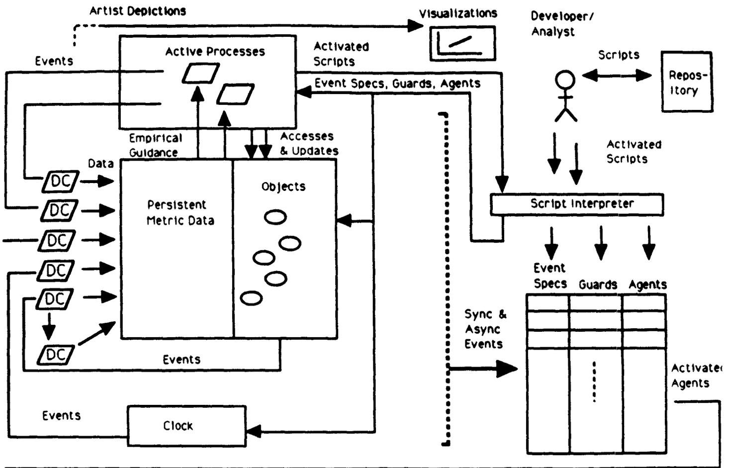
Figure 3: Conceptual operation of the *Amadeus* metric-driven analysis and feedback system.
