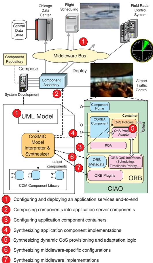
Figure 2: Incorporating Model-Integrated Computing with Component Middleware
