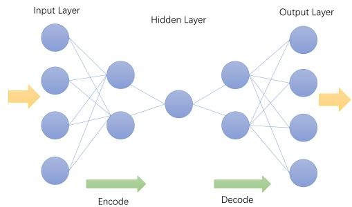
Fig. 6. Structure of Stacked Autoencoder.
