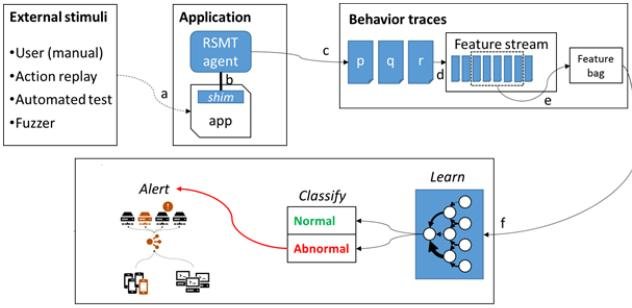
Fig. 1. The Workflow and Architecture of RSMT’s Online Monitoring and Detection System
