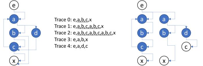
Fig. 3. Call Graph (L) and Call Tree (R) Constructed for a Simple Series of Call Stack Traces
