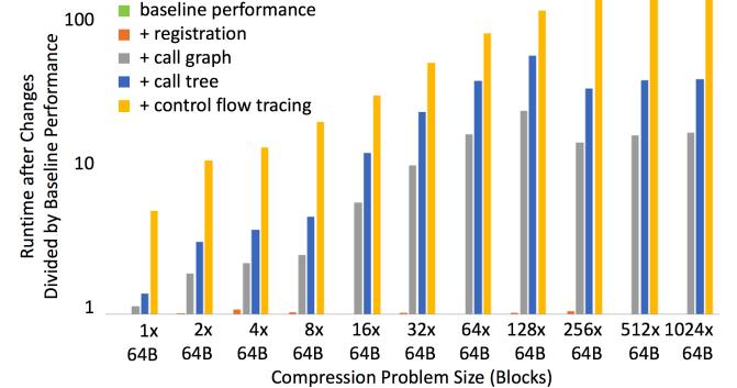
Fig. 10. Analysis of RSMT Performance Overhead
