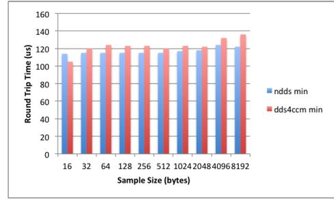
Figure 6: Ping Latency Minimum with Shared Memory
