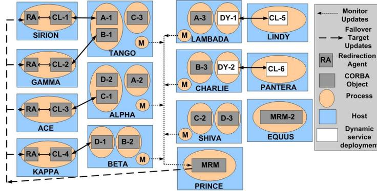
Fig. 2: Load-aware Failover Experiment Setup
