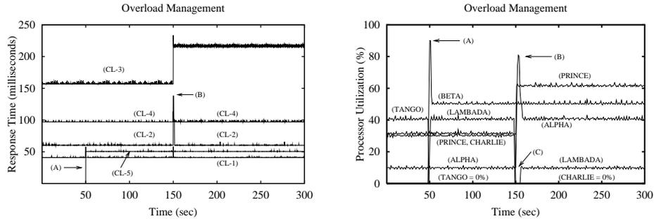
(a) Client response times with overload management (b) Utilizations with overload management
