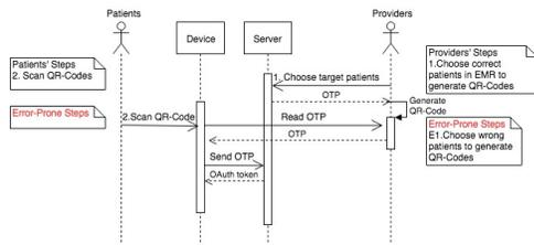
Fig. 4. Diagram of QR-Code based Authentication
