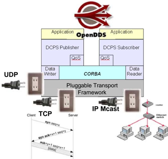
Figure 4: OpenDDS and its Transport Protocol Framework
