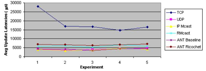
Figure 11: Baseline Emulab Experiment: 3 data readers, 3% loss, 25 Hz update rate
