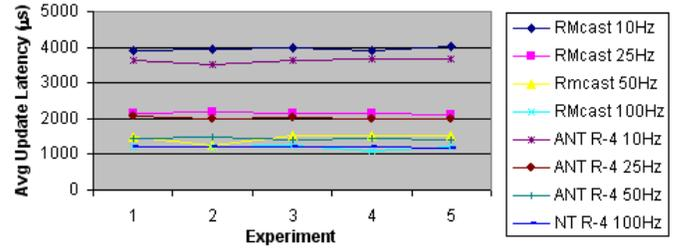
Figure 22: Latency ( $\mu s$ ) for ISISlab Experiment: 25 data readers, 1% loss
