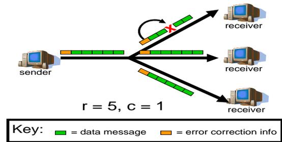
Figure 6: FEC Reliable Multicast Protocol - Sender-based
