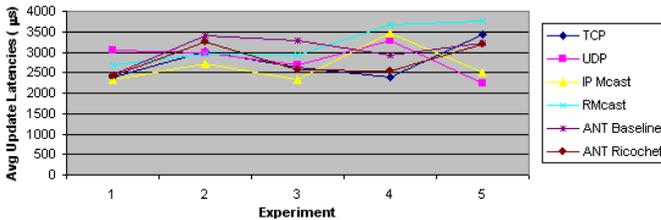
Figure 10: Baseline Emulab Experiment: 3 data readers, 0% loss, 50 Hz update rate
