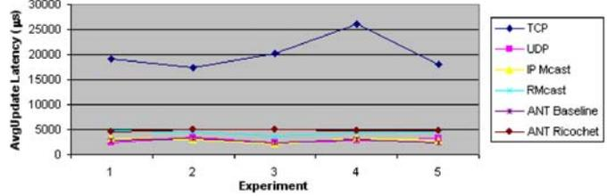
Figure 12: Baseline Emulab Experiment: 3 data readers, 3% loss, 50 Hz update rate
