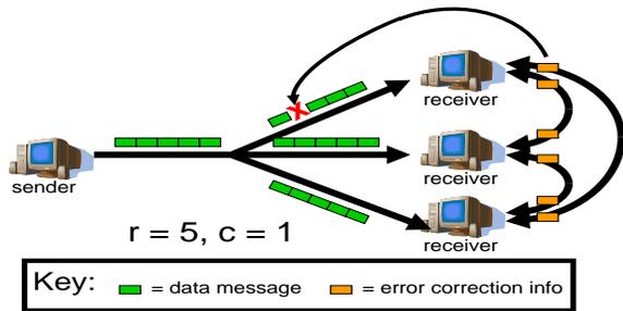
Figure 7: FEC Reliable Multicast Protocol - Receiver-based (LEC)
