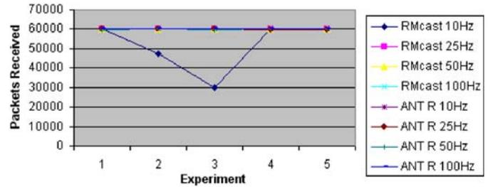
Figure 17: Packets Received for ISISlab Experiment: 3 data readers, 1% loss
