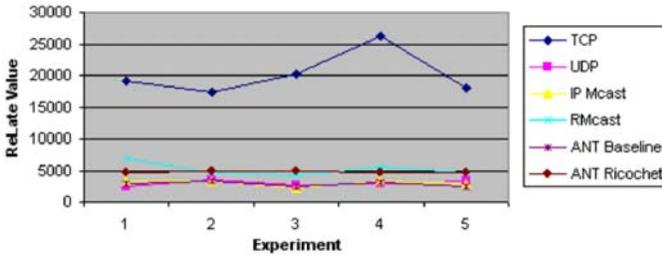
Figure 14: ReLate Metrics for Emulab Experiment: 3 data readers, 3% loss, 50 Hz update rate
