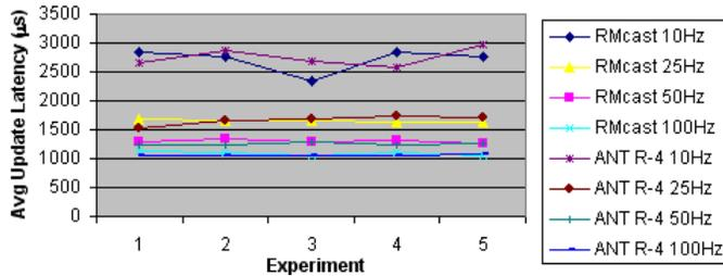
Figure 19: Latency ( $\mu s$ ) for ISISlab Experiment: 3 data readers, 1% loss
