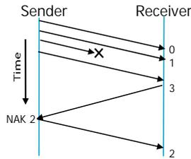
Figure 5: A NAK Based Protocol Discovering Loss
