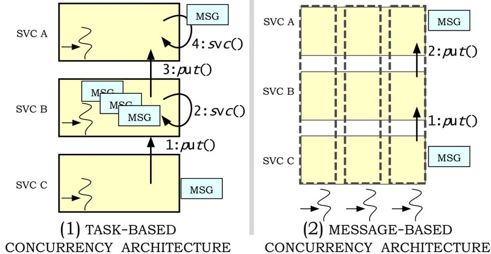
Figure 12: Alternative Methods for Invoking `put` and `svc` Methods
