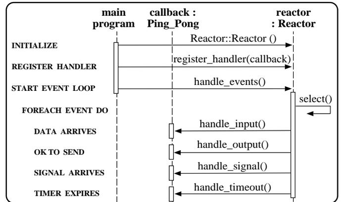
Figure 7: ACE Reactor Interaction Diagram
