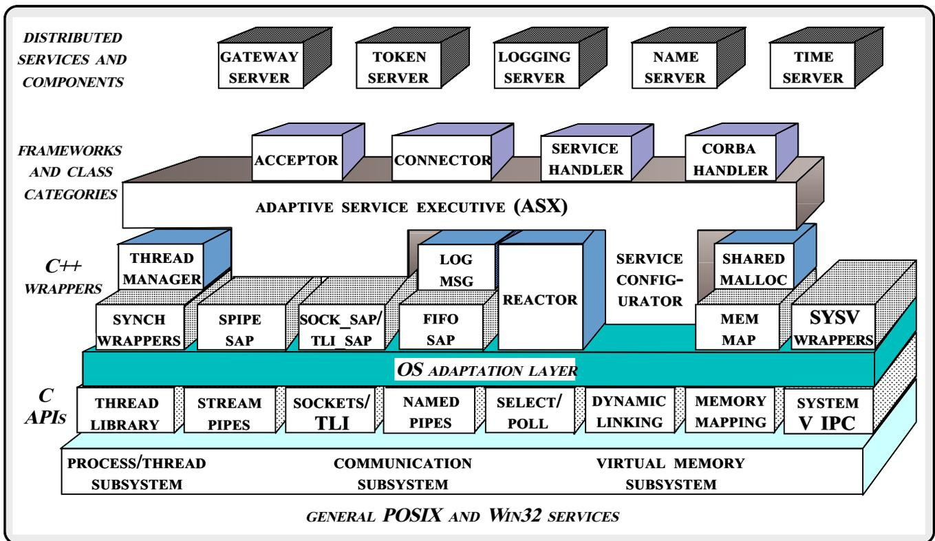
Figure 1: Components in the ADAPTIVE Communication Environment
