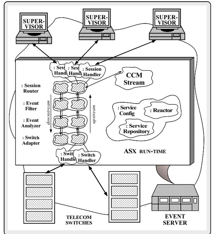
Figure 17: ASX Components for the PBX Application
