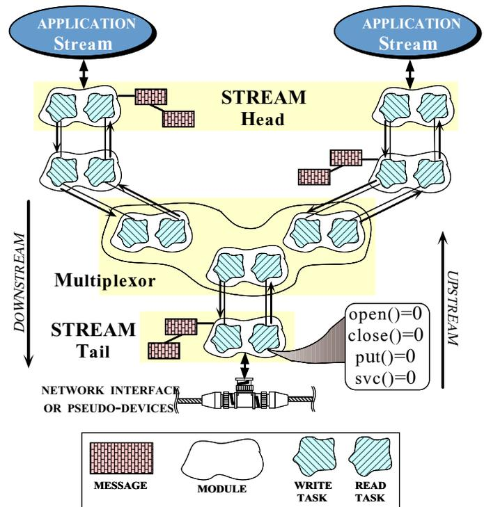
Figure 11: Components in the ASX Framework
