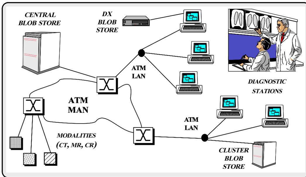
Figure 1: Topology of a distributed electronic medical imaging system.
