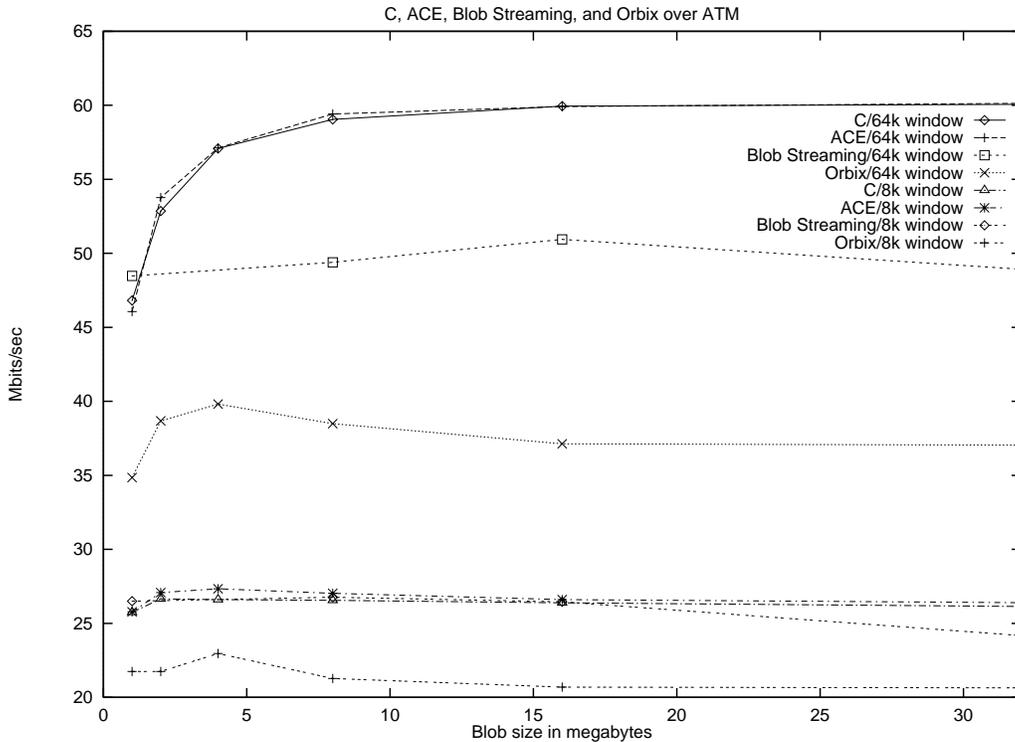
Figure 3: C, ACE C++, Blob Streaming, and Orbix performance over ATM.
