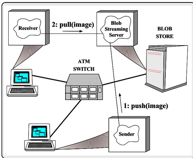
Figure 2: Push and pull models.
