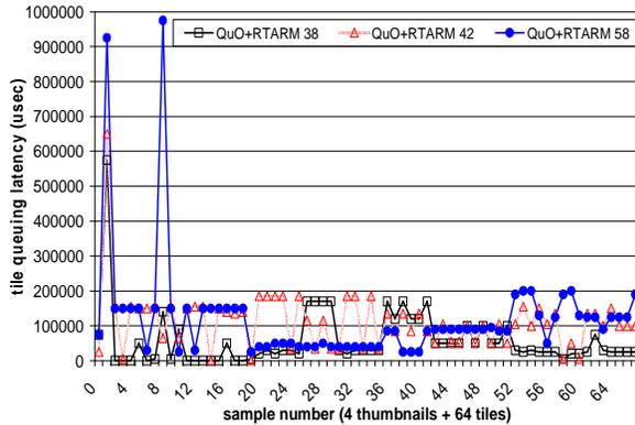
**Figure 13: Tile Queuing Latency with Adaptation**
