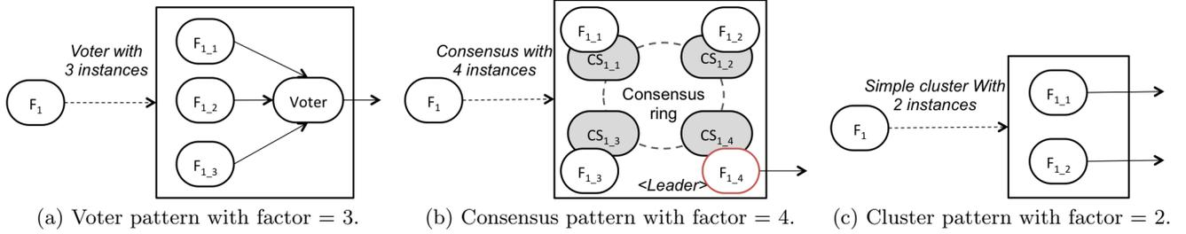
Figure 9: Example Redundancy Patterns for Functionality  $F_1$ . The  $CS_{n,m}$  entities represent consensus service providers.
