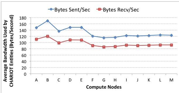
Figure 17: Average Network Bandwidth Consumption.
