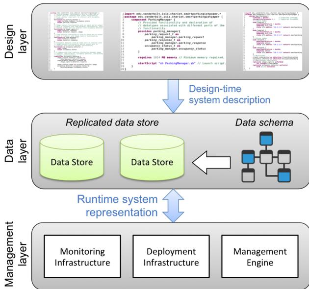
Figure 1: The Layered Architecture of CHARIOT.
