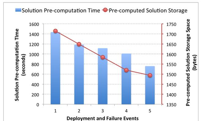
Figure 15: Solution Pre-computation Time for CPC with LaRC. (The solution for failure event  $i+1$  is computed when the reconfiguration action for the failure event  $i$  is being applied.)
