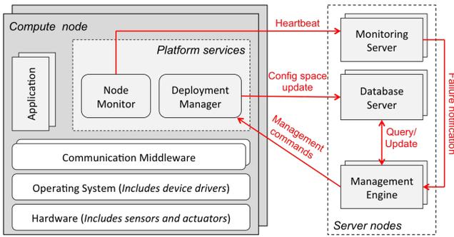
Figure 13: The Implementation Design of the CHARIOT Runtime.
