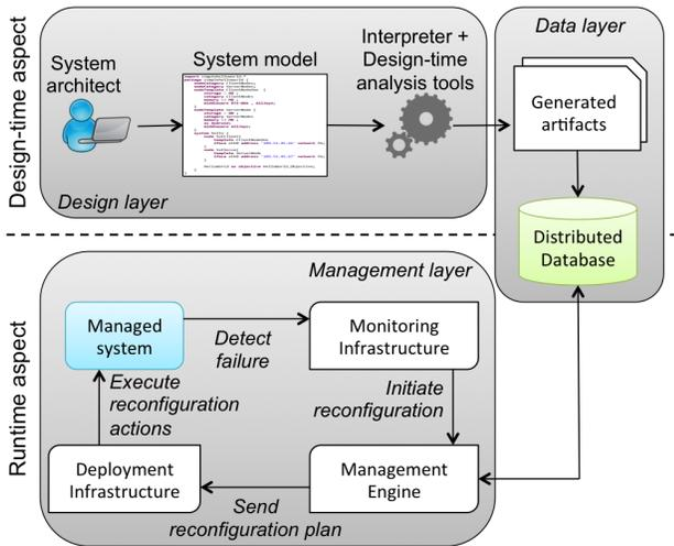
Figure 4: Overview of the self-reconfiguration mechanism.
