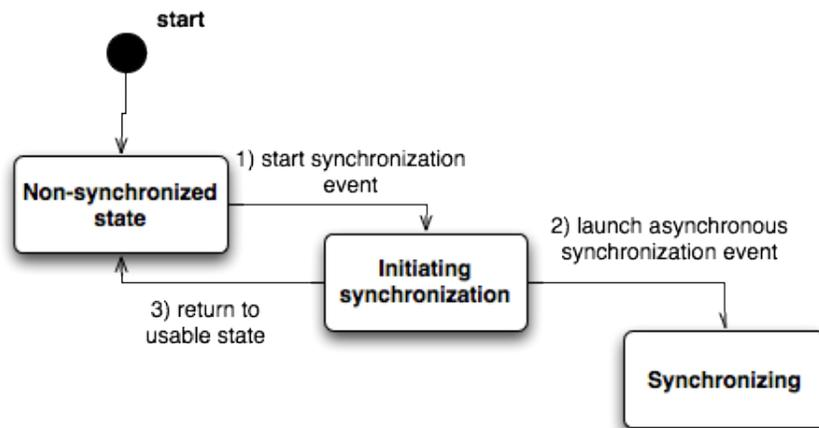
The *Asynchronous Data Synchronization* pattern is a mechanism pattern, thus it may be best visualized as a series of states. When an application is “usable” (meaning the user can interact with the application) a synchronization event can be started. Rather than executing the synchronization event sequentially, however, the event is launched asynchronously and the application returns to a usable state immediately.
