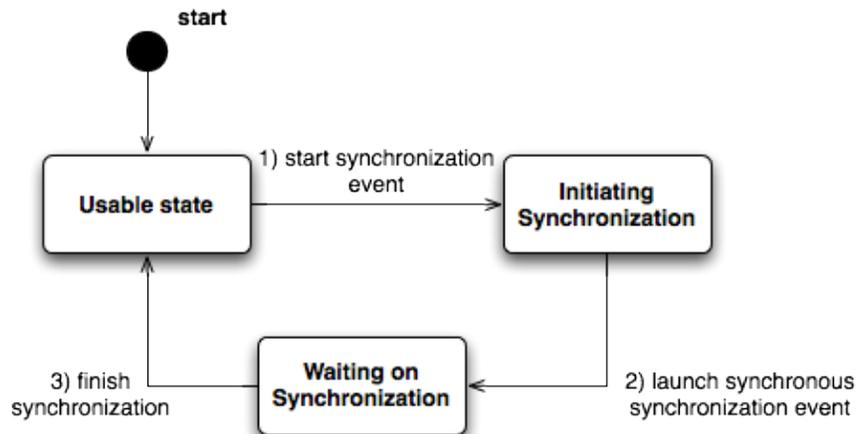
The *Synchronous Data Synchronization* pattern is a mechanism pattern as well, thus we will visualize it as a series of states. When an application is in a usable state, a synchronization event can be started. The event is launched synchronously and executed in a sequential fashion, leaving the application in a waiting state until the synchronization is finished, whereupon it returns to the usable state.
