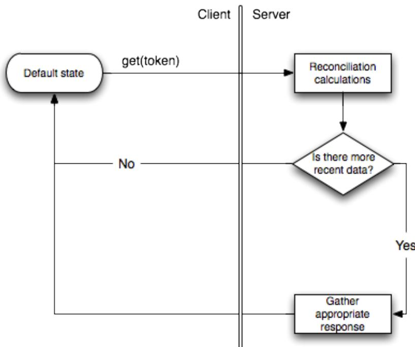
This flow chart is similar to the one in *Timestamp Transfer* with the addition of a process to calculate the differences in the data sets. In *Timestamp Transfer*, this is simply a comparison, but in *Mathematical Transfer*, this could be a more significant calculation that should be considered a separate process.
