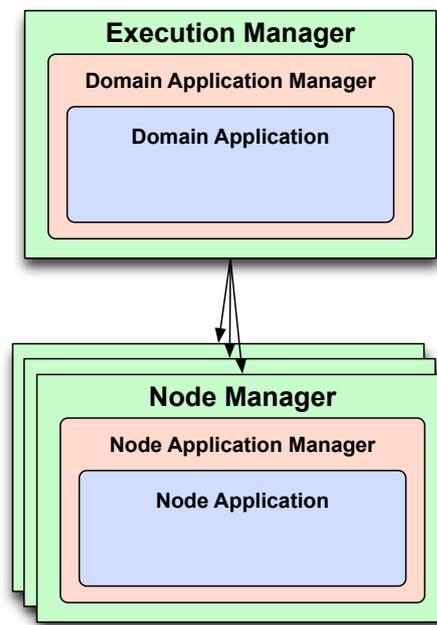
Figure 1.1: OMG D&C Architectural Overview and Separation of Concerns
