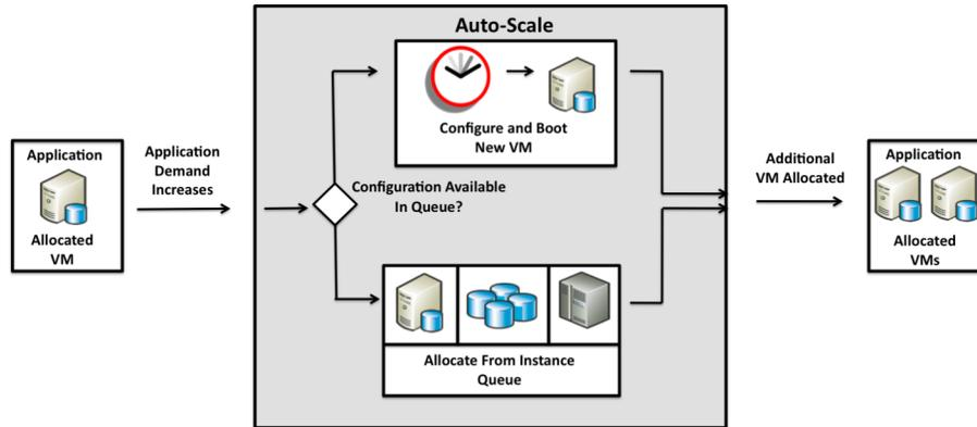
Fig. 1: Auto-scaling in a Cloud Infrastructure
