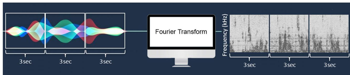
Fig. 1. To standardize input into the neural network, acoustic signals were segmented into 3-second chunks (left) and transformed into spectrograms using the Fourier transform (middle). Spectrograms displayed frequency over time, with intensity coded by grayscale (right).
