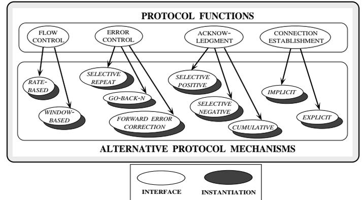
Figure 2: Protocol Functions and Protocol Mechanisms
