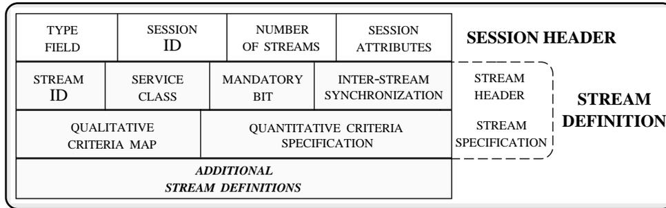
Figure 10: Structure of a Service Primitive
