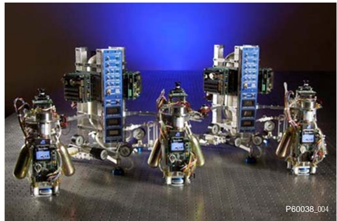
Figure 7 - The ATC Microbots and Picobots provide 2-D hardware simulation of spacecraft
