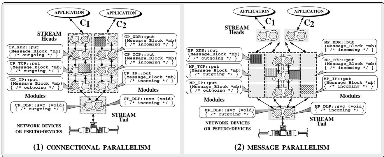
Figure 4: Message-based Process Architectures
