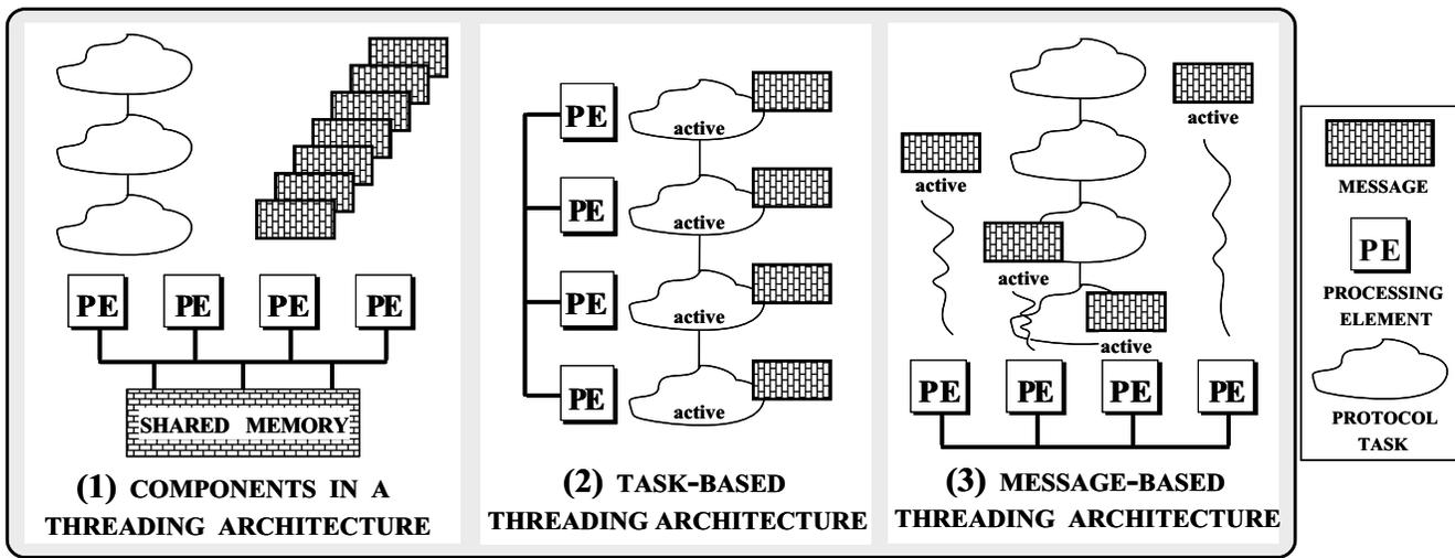
Figure 1: Basic Process Architecture Components and Interrelationships
