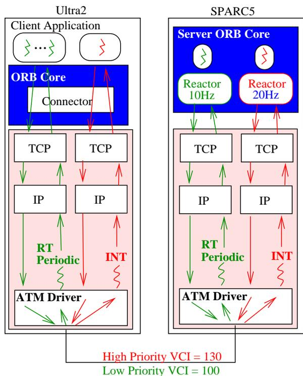
Figure 5: ORB Endsystem Benchmarking Configuration
