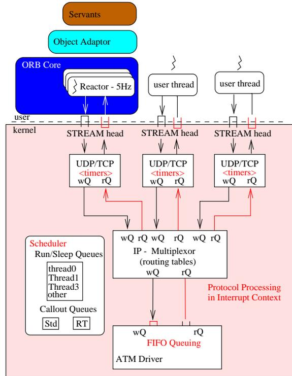
Figure 10: Conventional Protocol Stacks in Solaris STREAMS
