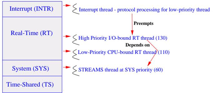
Figure 2: Common Sources of Priority Inversion in Solaris
