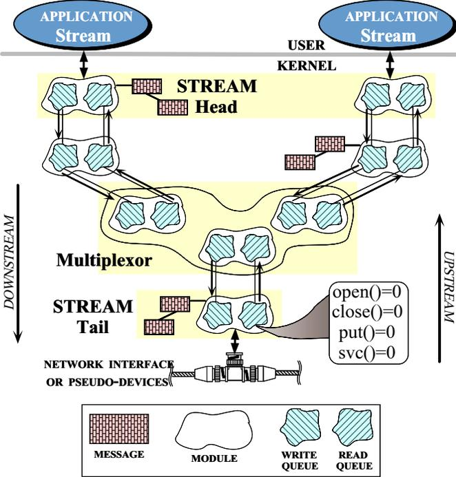
Figure 9: General Structure of a STREAM
