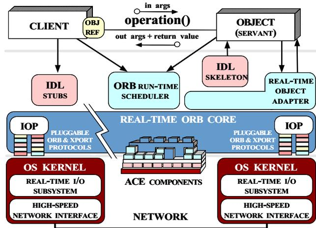
Figure 1: Components in the TAO Real-time ORB Endsysteem
