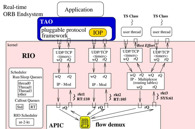
Figure 3: Architecture of the RIO Subsystem and Its Relationship to TAO
