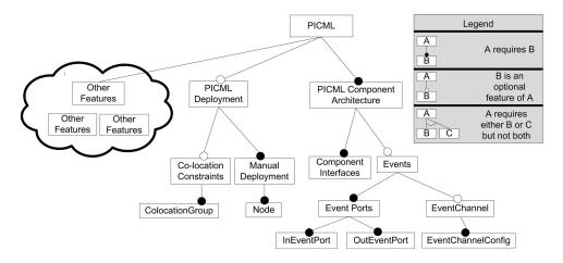
Figure 2. PICML Feature Model Snippet for Event Elements
