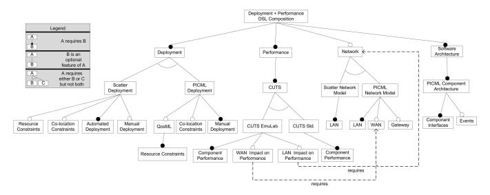
Figure 3. A Feature Model for the PICML/CUTS/Scatter/CQML DSL Family
