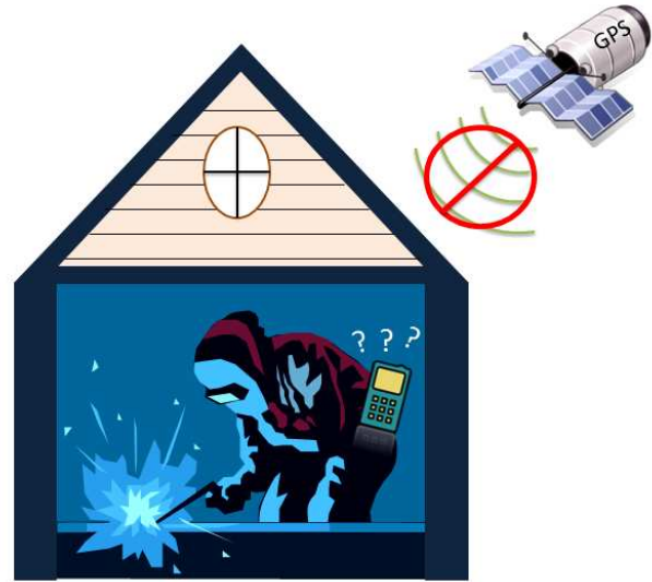
Figure 2. GPS Signals Blocked in a Construction Environment
