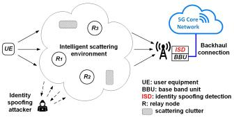
Fig. 3. Conceptual system setting with intelligent scatting environment (ISE)
