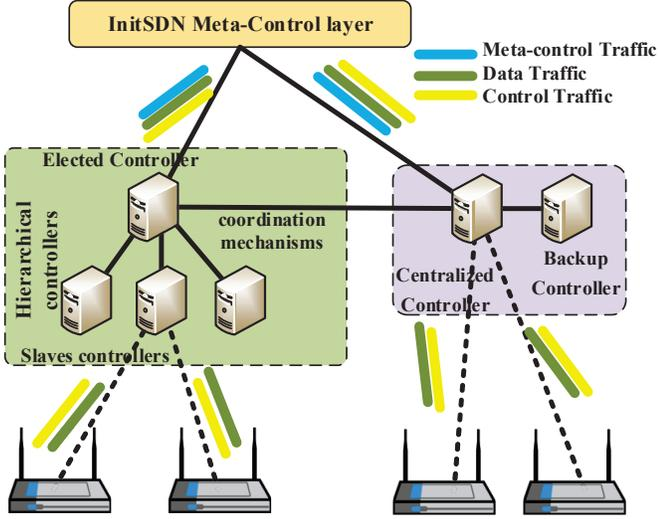
Fig. 3: InitSDN Hybrid Control Plane for the STLS
