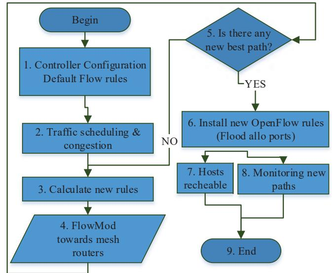
Fig. 4: The framework for the load balancer
