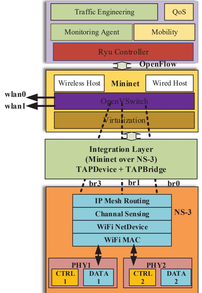
Fig. 2: Design of the OpenFlow-enabled mesh router
