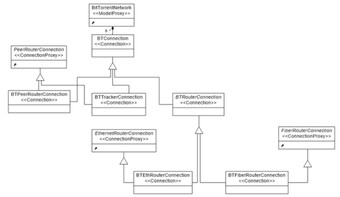
Fig. 10: Metamodel of BitTorrent Network Connection
