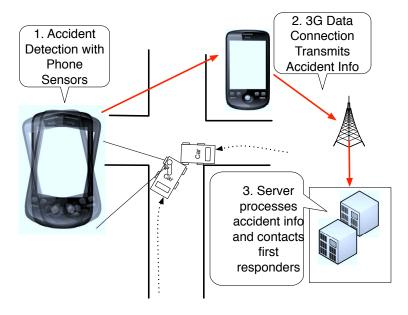
Fig. 2: Smartphone-Based Accident Detection System
