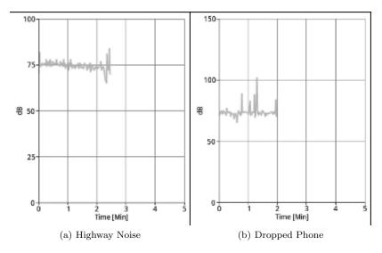
Fig. 9: Potential Noise Levels During Highway Transportation
