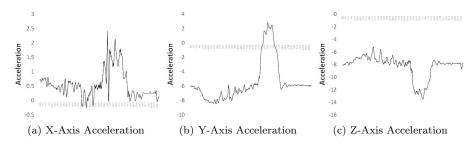
Fig. 13: Acceleration During a Sudden Stop
