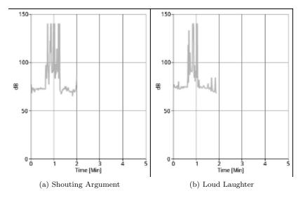
Fig. 10: Human Noise Levels During Highway Transportation
