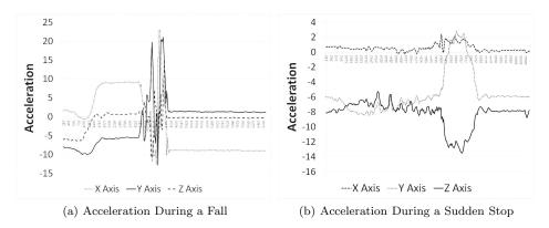
Fig. 8: Acceleration During Falls and Sudden Stops
