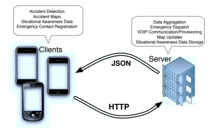
Fig. 3: WreckWatch Architecture Diagram
