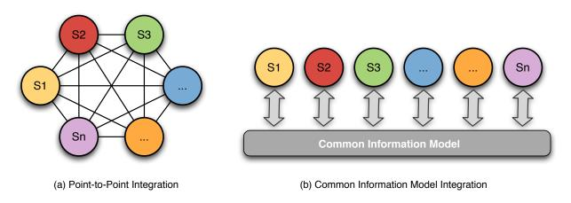
Figure 8: System of System Integration Styles.
