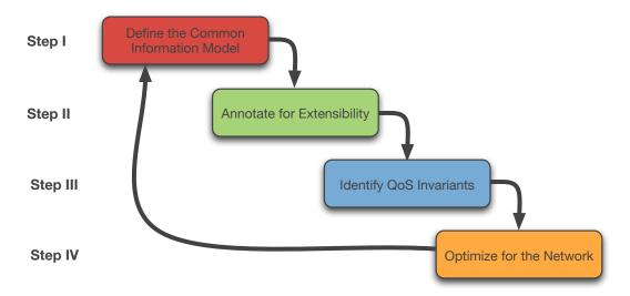
Figure 7: Visual representation of the steps involved in the common information model approach.
