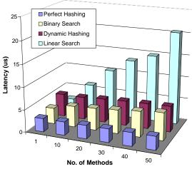
Figure 10: Operation Demultiplexing Latency with Alternative Search Techniques
