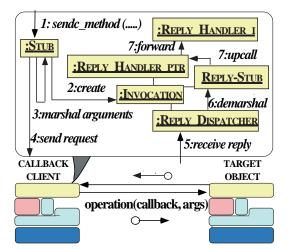
Figure 11: Client ORB Interactions for an Asynchronous Twoway Operation
