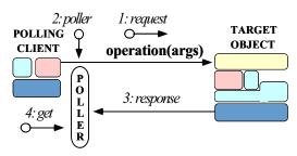
Figure 1: Polling Model for CORBA Asynchronous Twoway Operations
