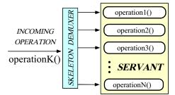
Figure 8: Operation Demultiplexing in Skeletons
