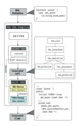
Figure 5: Interactions Between Internal Components in TAO's IDL Compiler
