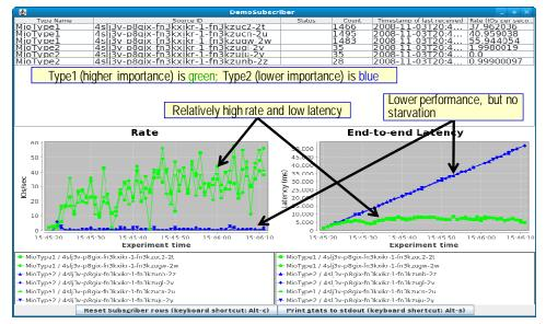
Figure 8. The QoS GUI Displays the Client-visible Behavior Under QED control, including Throughput and Latency
