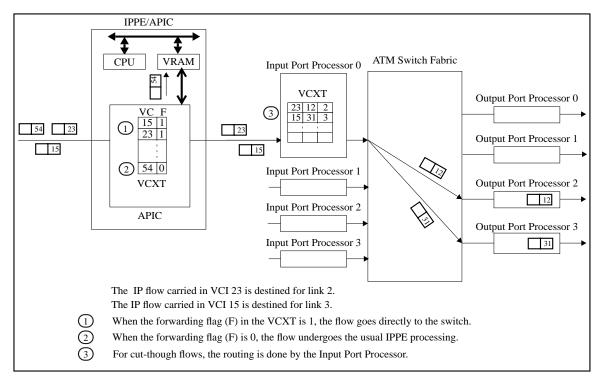
Figure 6: Cut-through Routing
