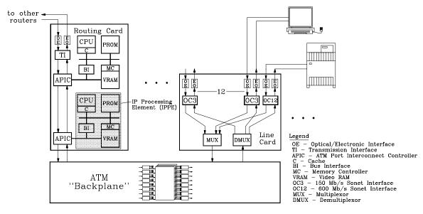
Figure 1: Gigabit a<sup>I</sup>t<sup>P</sup>m Router
