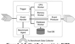
Figure 5. A CoWorkEr Assembly in CUTS
